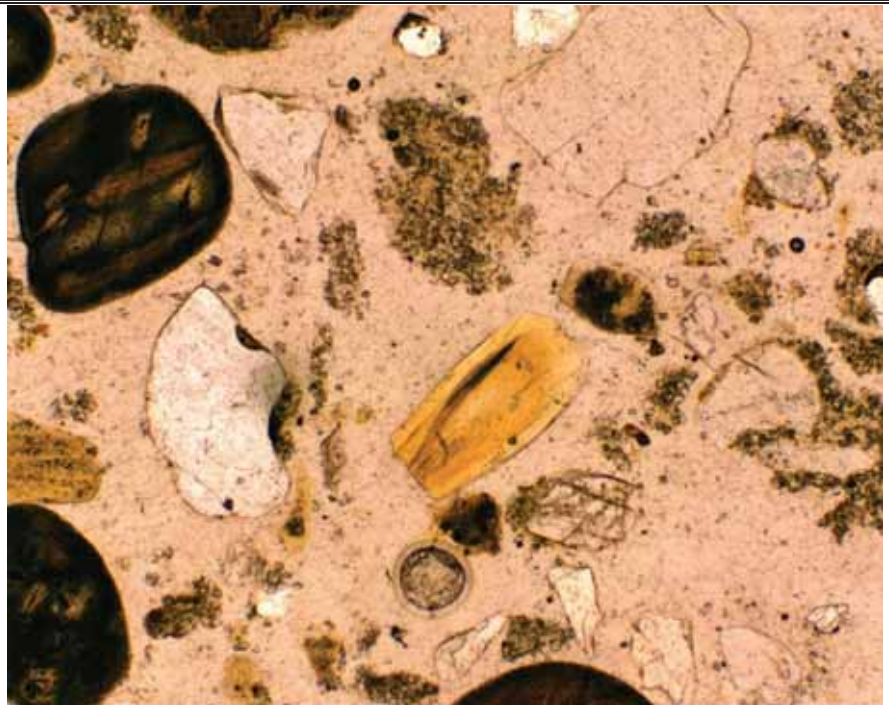
Phosphatic bone fragment and collophane "balls" in a dolomitic, clay-rich matrix (brown). Polarized light.
